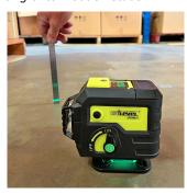
Laser Output (H/V): Green Class 3r 500nm - 550nm <5mW
