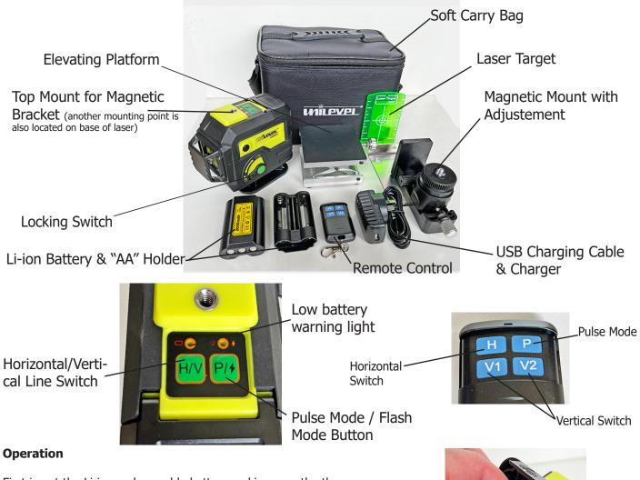
First insert the Li-ion rechargeable battery making sure the three terminal are facing inside the battery compartment. The battery is charged using the supplied charger or any USB A output. To charge remove battery from the laser and plug directly into the battery. Alternatively you can charge the battery inside the unit using the USB C socket below the battery compartment. You can also use standard "AA" batteries if required with the standard battery holder.
