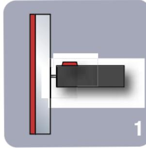
When the sensors are not in contact with the low-e coating no audible tone will be heard.
