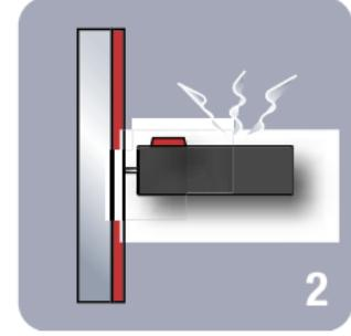
When the sensors are in contact with the low-e coating an audible tone will be emitted from the detector to indicate its presence.
