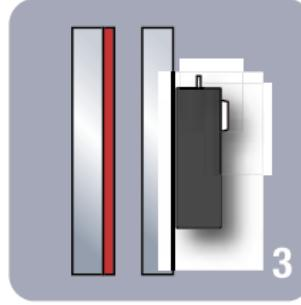
If the tool does not detect the presence of a low-e coating on the piece of glass that the tool is touching no audible tone will be emitted. If no tone is emitted simply repeat this procedure on the opposite side of the unit as shown below.
