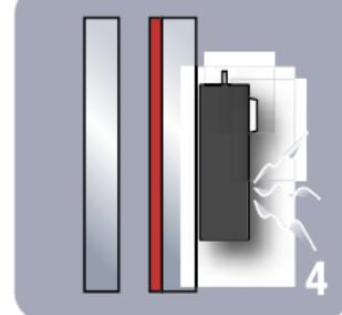
If the tool detects the presence of a low-e coating on the piece of glass that the tool is touching an audible tone will be emitted to indicate this.
