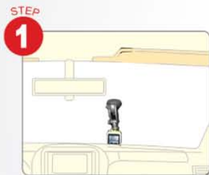
1. Attach DVR-6330 to the car windscreen with supplied mounting.
