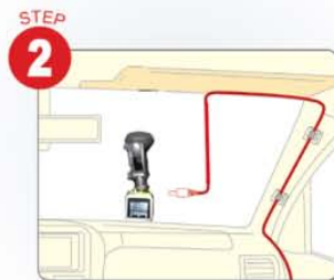
2. Plug DVR-6330 car charger to working cigarette lighter and hook the hang down line with wire clips.
